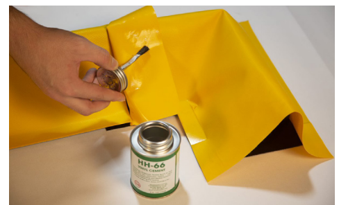
Attach corners using vinyl cement.
